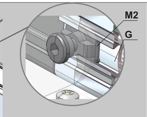
5) Fig.12a- Make sure that the actuator rod has completely retracted into the actuator.
